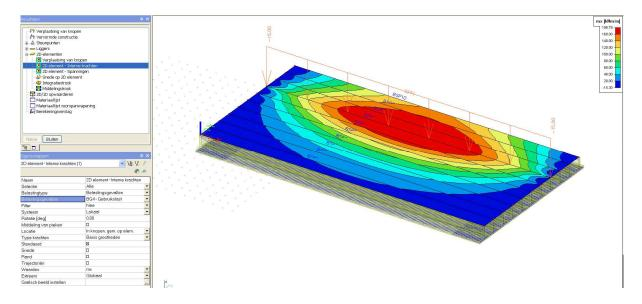
There is a clear spreading noticeable. The local line load of 15kN/m will be spread over multiple beams. This spreading is caused by the transversal stiffness of the prefab plate model. This transversal stiffness will be delivered by the in situ topping of the bridge deck (and not by the prefab beam elements themselves who will serve of course for the longitudinal stiffness).
