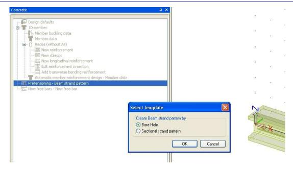
The bore hole pattern will be defined on a profile. We choose of course the above defined cross-section. The definition of the bore hole pattern can be done by means of the input of individual holes or a whole region.
