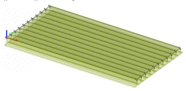
It is also possible to define the prestress reinforcement in this model, but it will not be taken into account for the calculation. It will however be exported to the 1D elementmodel where it will be taken into account in the analysis.
