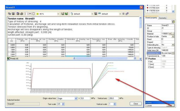
In this example a transmission length of 1m is entered. Also no additional losses like an anchorage set loss or a short term relaxation loss are taken into account. They could be defined by means of the advanced parameters, but they are not treated in this example. (To have access to these parameters the functionality prestressing>advanced needs to be ticked on.)
