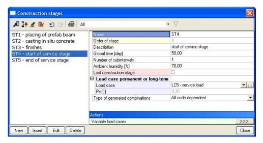
The Psi factor of 0,3 will only influence the participation of LC5 to the long term losses calculated by TDA solver. In the generated combinations, this load case will be considered without this reduction factor, so this reduction factor is only for the calculation of losses, not for the concrete checks.
