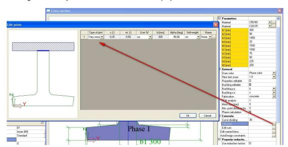
The roughness of the joint can be defined in the section properties:
