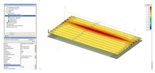
To increase the spreading of the loads, a transverse beam could be added to the model.
