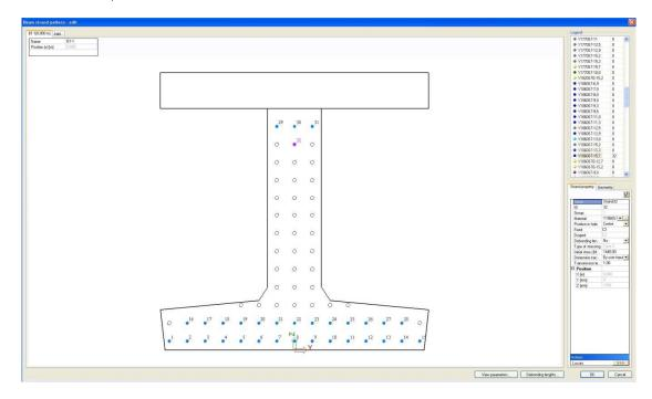
The top strands are bent so they will join the bottom strands at a distance of 3m from the support. To achieve this an extra section at 3m is created and on this section a drape of 800mm is given to the top strands.
