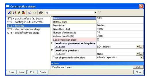
Note that stage 3 is the last construction stage.
