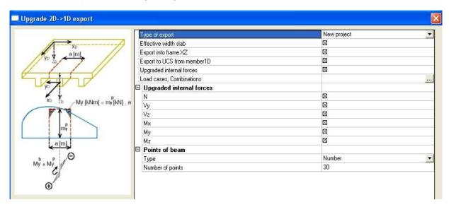
The width of bridge deck that is taken into account in the export is defined by the effective width (which could be enterred in the properties of the prefab slab). This effective width is also used as integration width to define the equivalent internal forces on the 1D element model.
