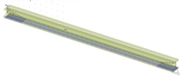
To edit the properties afterwards, the beam strand pattern should be selected. Trough the property menu the user can click on edit strand pattern to edit the strand pattern at any time.
