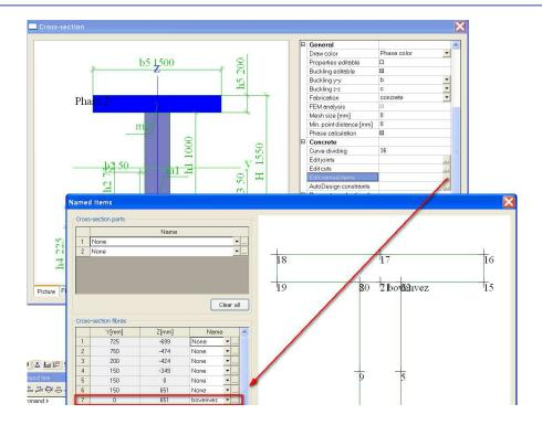
Afterwards stresses can be shown over this named fibre. In the picture below the stress in stage 5 on the top fibre of the precast beam is shown:
