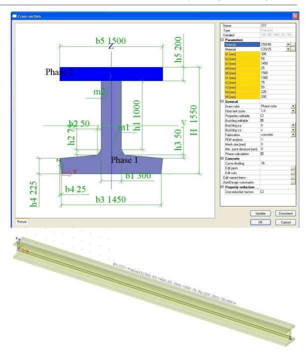
The input of the pretensioning is done in the concrete menu.
