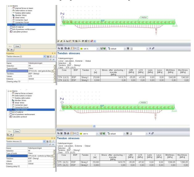
There is clearly an increase in LCS losses between the beginning and the end of the service stage.
