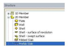
The prefab slab will be considered as a 'normal' plate in this 2D element model.
