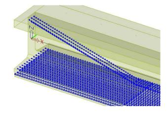
It is already possible to have a look at the stress after transfer that is put to the beam before the construction stage analysis is run. This can be accessed through the action menu below the properties of a strand.
