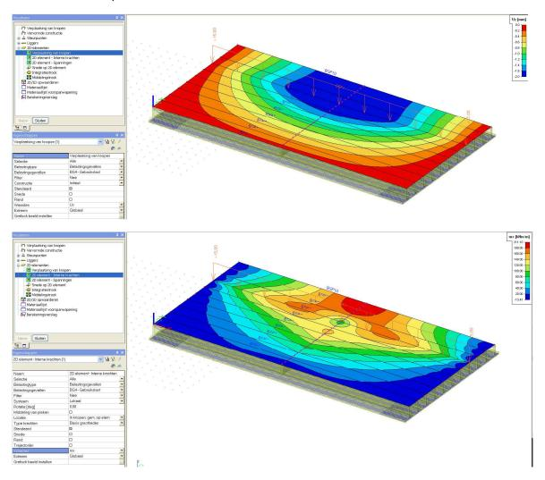
The transverse beam is clearly providing a better spreading of the loads.
