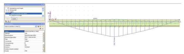
This moment line is a result of integration from the internal forces on the 2D prefab slab model.
